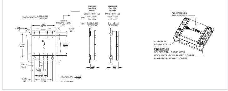
Figure 10 — PCB mounting specifications
