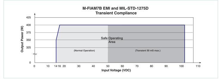
Figure 7 — M-FIAM7B EMI and MIL-STD-1275D transient compliance
