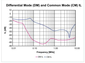
Figure 5 — Insertion loss curve
