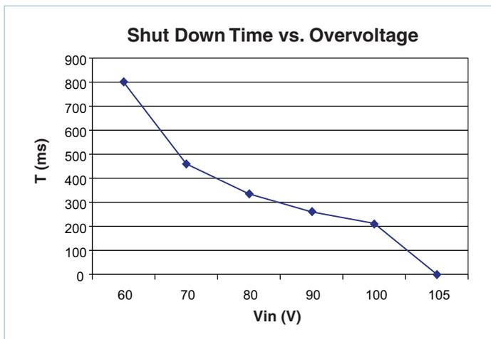
Figure 1 —  $T$  = time period before overvoltage protection.
