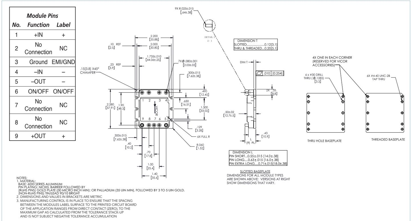
Figure 9 — Mechanical diagram
