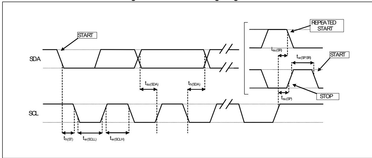
Note: Measurement points are done at 0.2·Vdd\_IO and 0.8·Vdd\_IO, for both ports.
