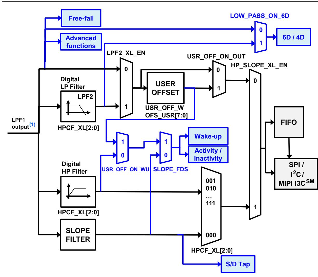
1. The cutoff value of the LPF1 output is ODR/2 when the accelerometer is in high-performance mode and ODR up to 833 Hz. This value is equal to 780 Hz when the accelerometer is in low-power or normal mode.
