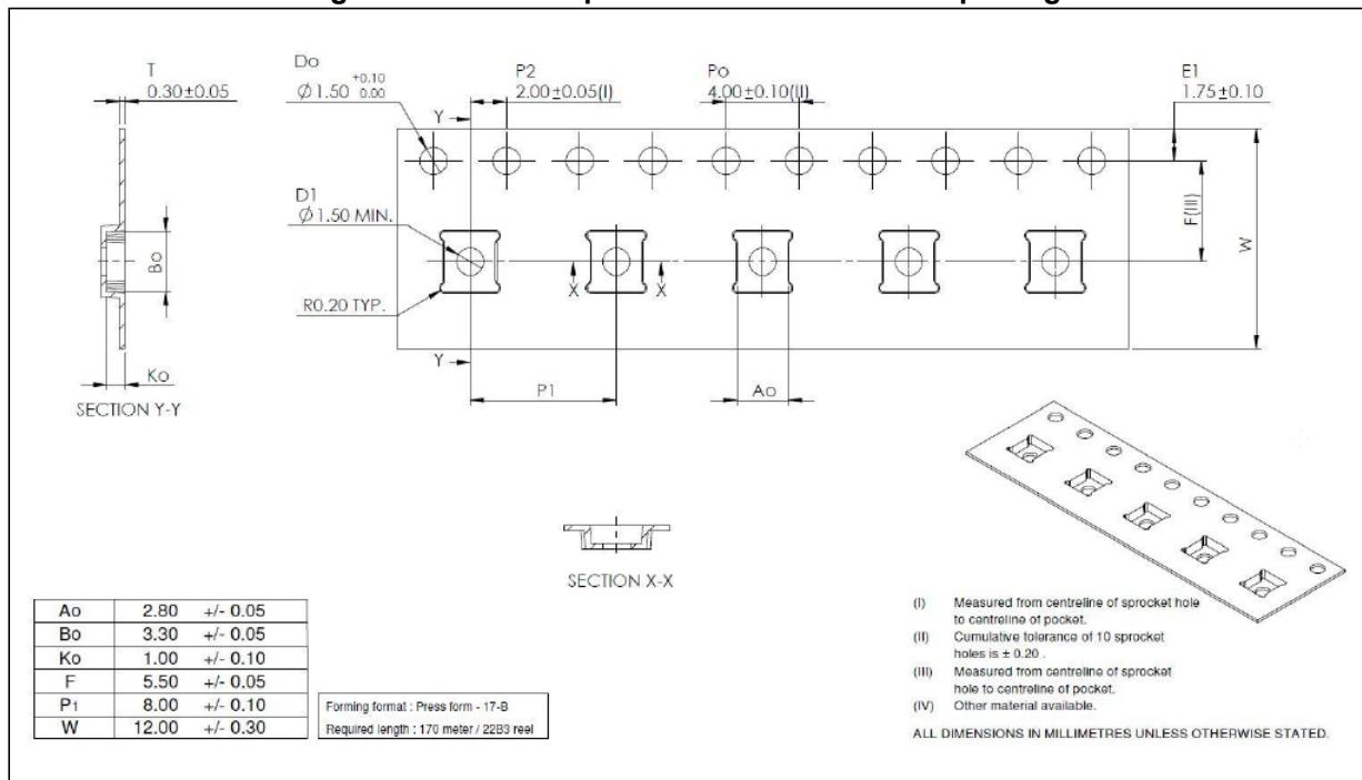
Figure 28. LGA-14 package orientation in carrier tape
