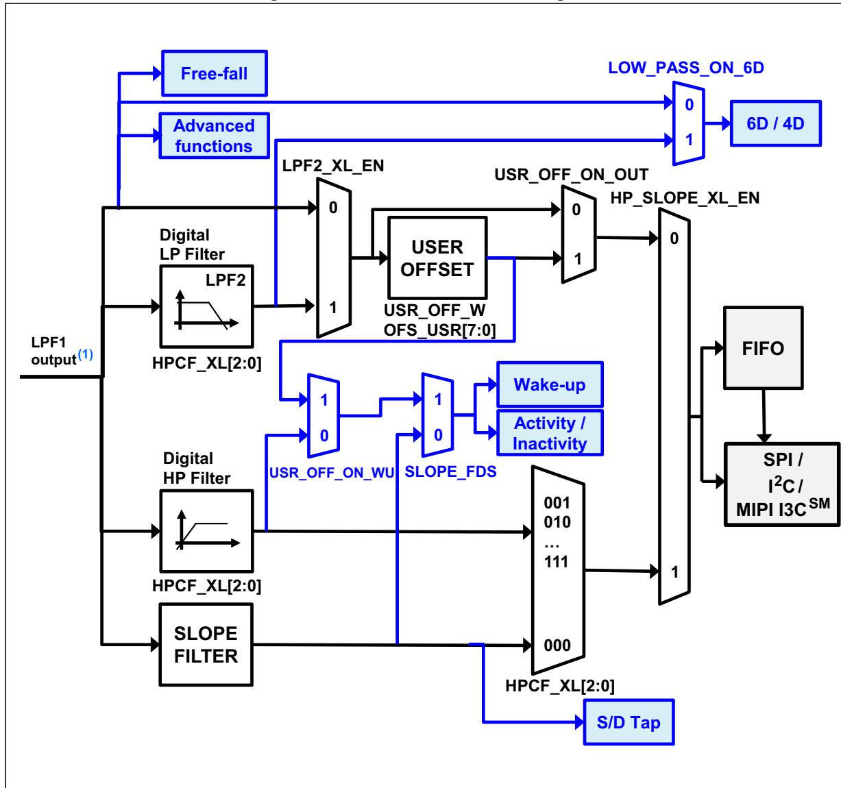
1. The cutoff value of the LPF1 output is ODR/2 when the accelerometer is in high-performance mode and ODR up to 833 Hz. This value is equal to 780 Hz when the accelerometer is in low-power or normal mode.
