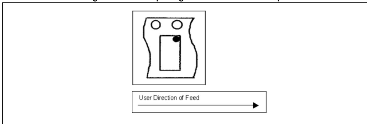
**Figure 29.** Reel information for carrier tape of LGA-14 package
