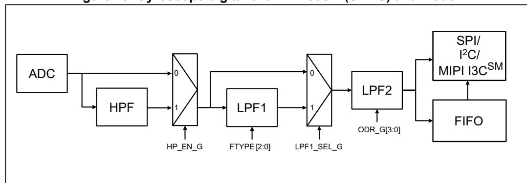
In this configuration, the gyroscope ODR is selectable from 12.5 Hz up to 6.66 kHz. A low-pass filter (LPF1) is available if the auxiliary SPI is disabled, for more details about the filter characteristics see [Table 65: Gyroscope LPF1 bandwidth selection](#).
