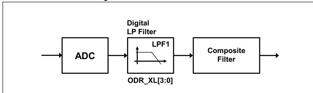
Figure 17. Accelerometer composite filter
