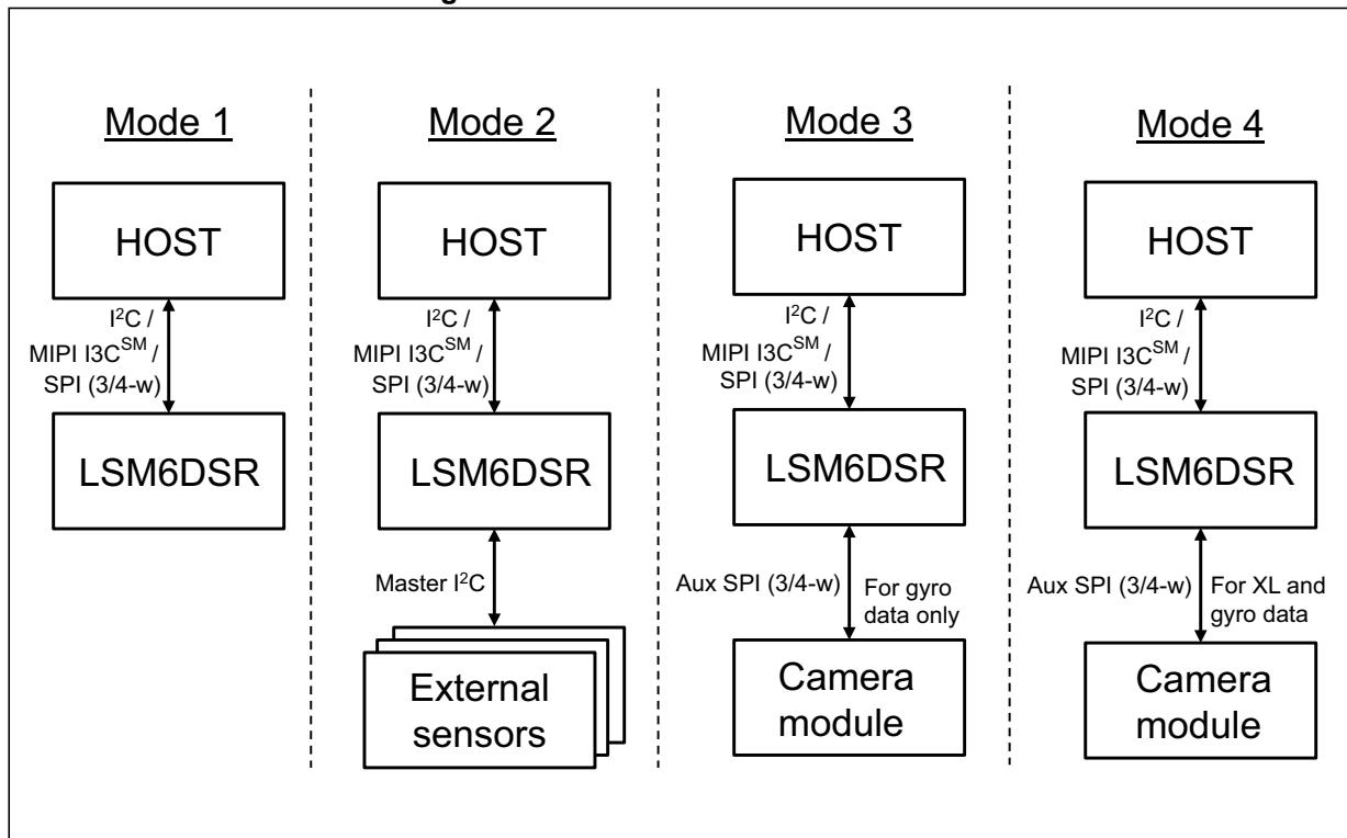
In the following table each mode is described for the pin connections and function.
