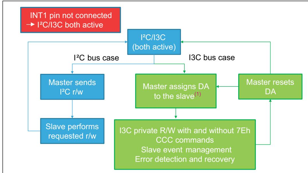
1. Address assignment (DAA or ENTDA) must be performed with I<sup>2</sup>C Fast Mode Plus Timing. When the slave is addressed, the I<sup>2</sup>C slave is disabled and the timing is compatible with I3C specifications.
