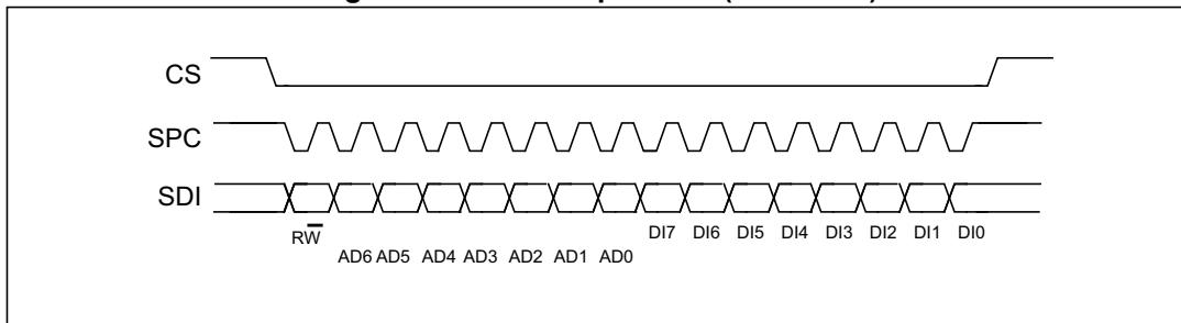
The SPI Write command is performed with 16 clock pulses. A multiple byte write command is performed by adding blocks of 8 clock pulses to the previous one.
