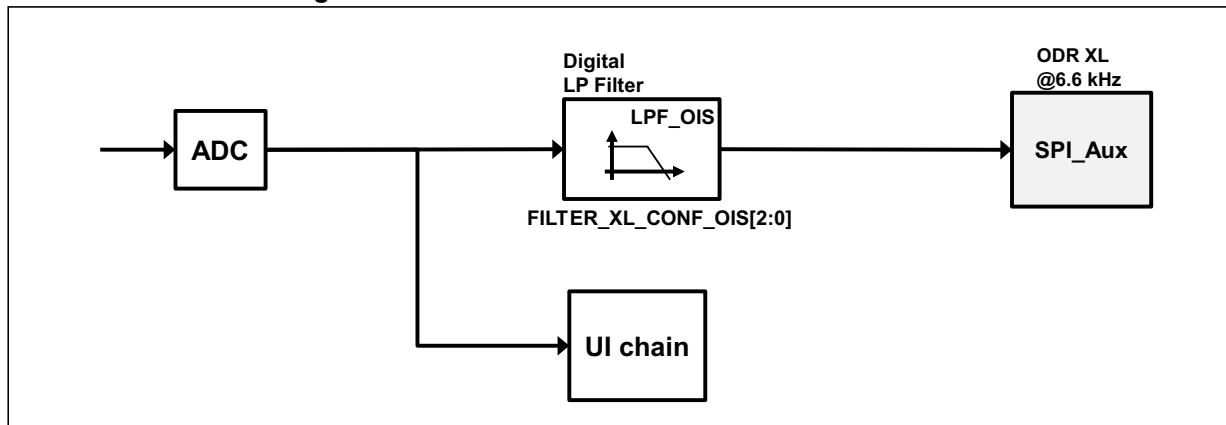
**Note:** Mode 4 is enabled when Mode4\_EN = 1 and OIS\_EN\_SPI2 = 1 in CTRL1\_OIS (70h).
