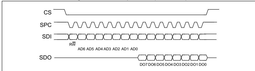
The SPI Read command is performed with 16 clock pulses. A multiple byte read command is performed by adding blocks of 8 clock pulses to the previous one.
