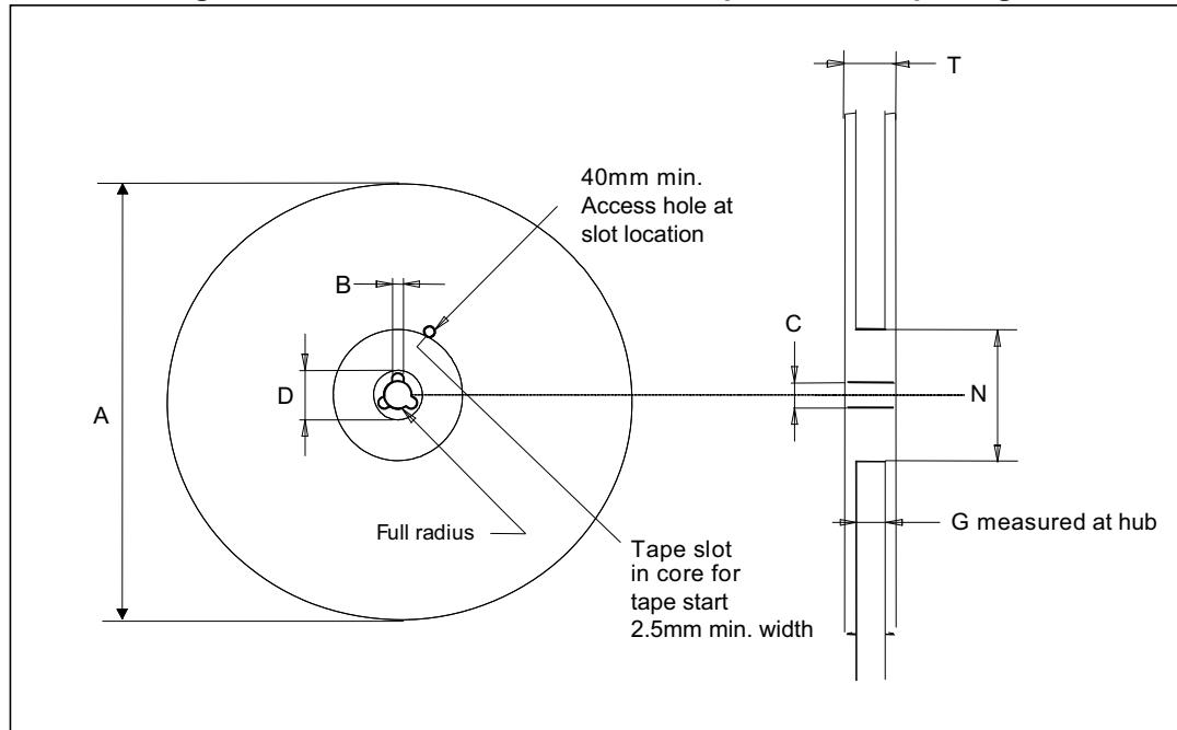
**Table 401.** Reel dimensions for carrier tape of LGA-14 package
