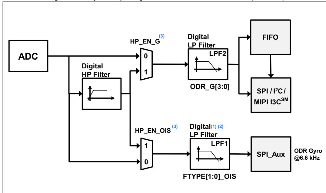
1. When Mode3/4 is enabled, the LPF1 filter is not available in the gyroscope UI chain.
