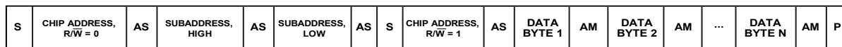
S = START BIT, P = STOP BIT, AM = ACKNOWLEDGE BY MASTER, AS = ACKNOWLEDGE BY SLAVE. SHOWS A ONE-WORD READ, WHERE EACH WORD HAS N BYTES.
