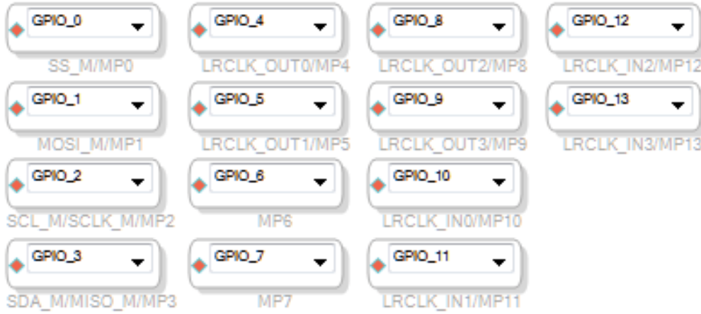
Figure 76. Complete Set of General-Purpose Outputs in SigmaStudio
