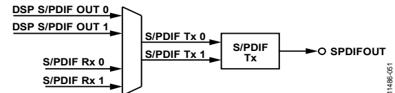
Figure 48. S/PDIF Transmitter Source Selection
