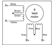
Eight lead motor connected to a unipolar drive.
