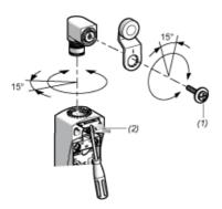
(1) Tightening torque (Min: 1) (Max: 1.5)
