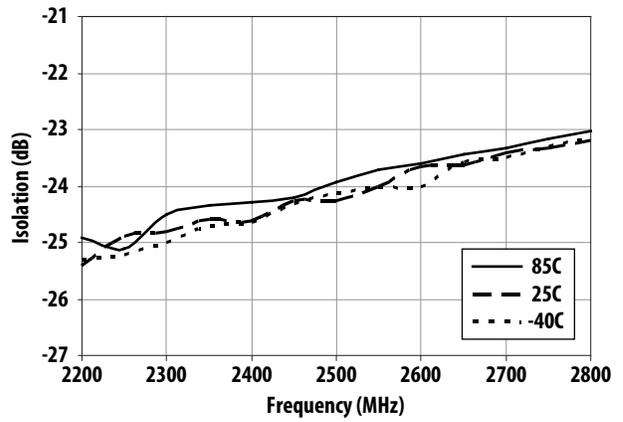
Figure 39. Isolation vs Frequency and Temperature
