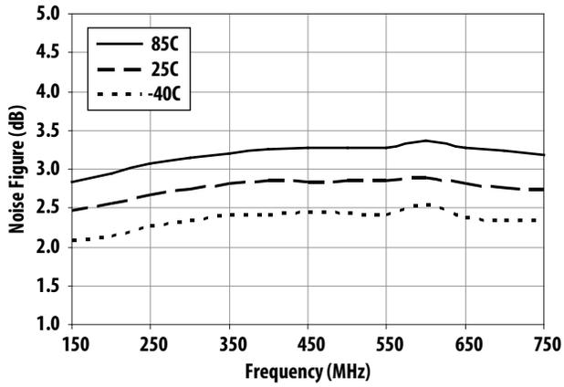
Figure 13. Noise Figure vs Frequency vs Temperature
