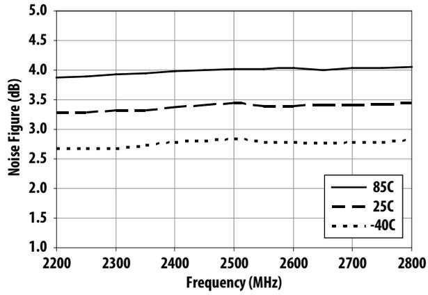
Figure 40. Noise Figure vs Frequency vs Temperature
