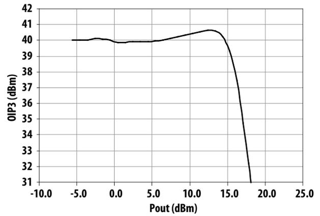
Figure 23. OIP3 vs Output Power at 1900MHz
