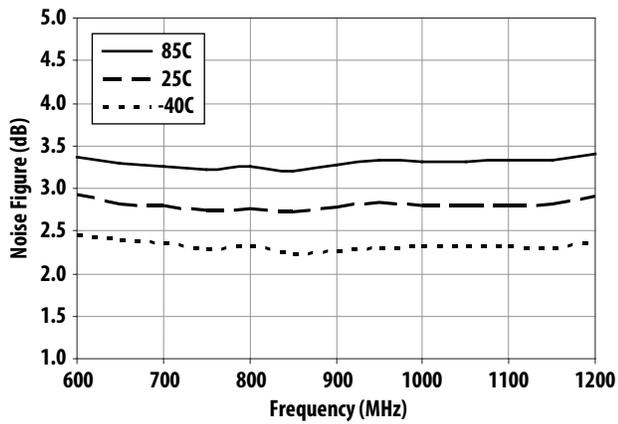
Figure 22. Noise Figure vs Frequency vs Temperature
