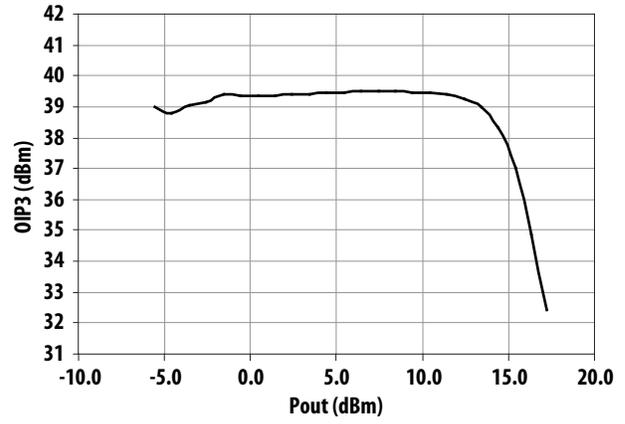
Figure 32. OIP3 vs Output Power at 1900MHz
