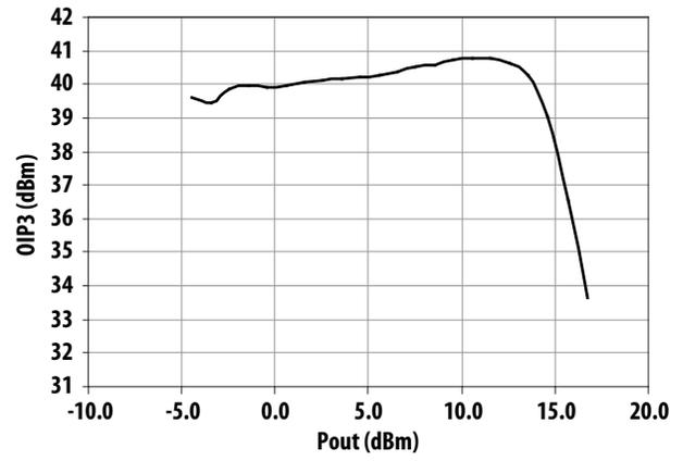
Figure 41. OIP3 vs Output Power at 1900MHz
