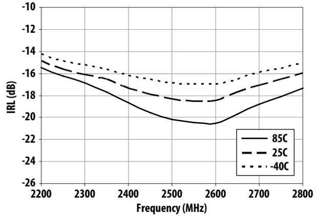
Figure 37. IRL vs Frequency and Temperature
