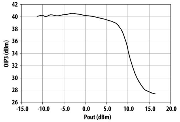
Figure 14. OIP3 vs Output Power at 450MHz
