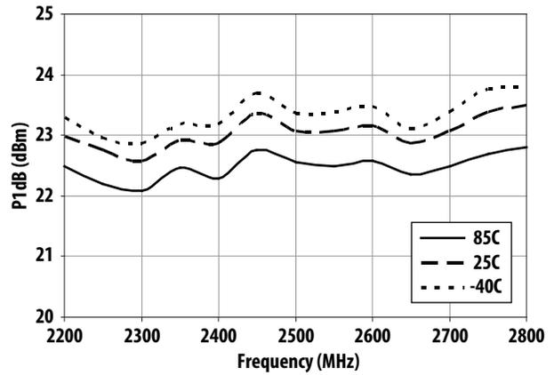
Figure 35. P1dB vs Frequency and Temperature
