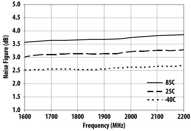
Figure 31. Noise Figure vs Frequency vs Temperature
