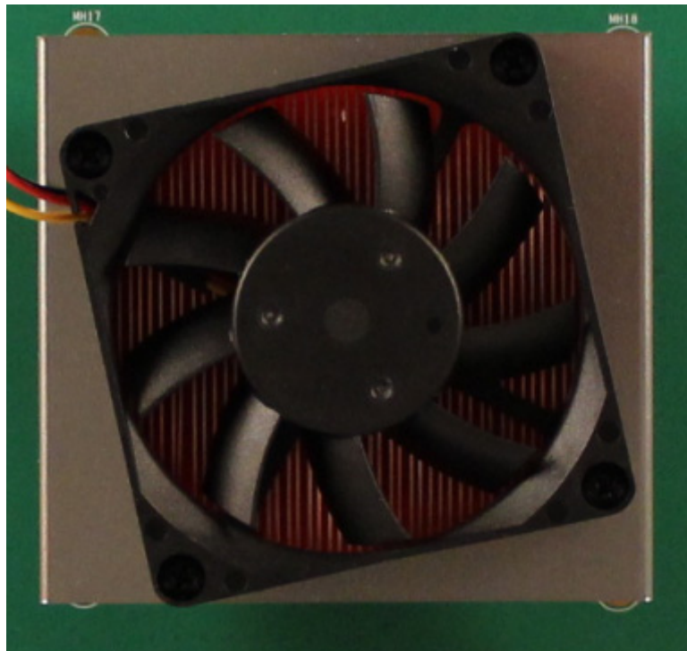
Figure 3-5: Active FPGA Heat Sink
