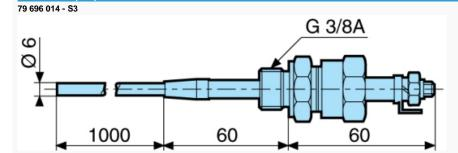
Electrode holder with a single probe supplied in a standard length of 1000mm. (304 stainless steel). Mounting with external 3/8" BSP thread and hexagonal head. Use 24 mm. spanner for hexagon. Suitable for use on boilers, autoclaves and under high temperature conditions up to 200 °C and high pressure conditions up to 25 kg/cm 2
