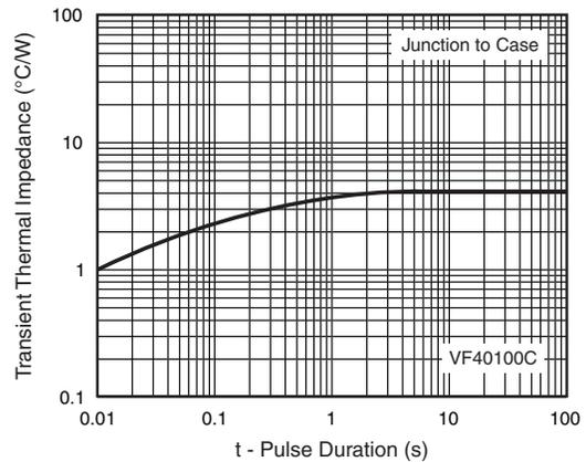
Fig. 7 - Typical Transient Thermal Impedance Per Diode
