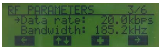
Figure 9. Menu Page: RF Parameters 3/6 (Modulation is OOK)
