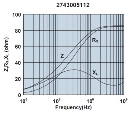
Impedance, reactance, and resistance vs. frequency.
