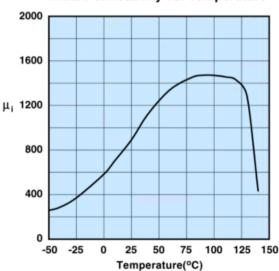
Measured on a 17/10/6mm toroid at 100kHz.
