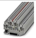
Component terminal block, Connection type: Spring-cage connection, Cross section: 0.08 mm² - 4 mm², AWG: 28 - 12, Nominal current: 22 A, Nominal voltage: 500 V, Length: 67.5 mm, Width: 5.2 mm, Color: gray, Assembly: NS 35/7,5, NS 35/15
