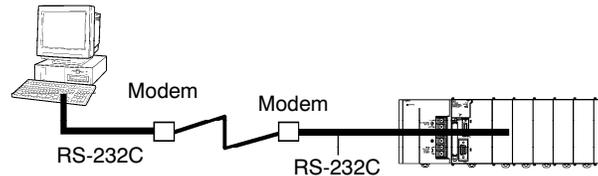
Monitoring and editing online from CX-Programmer for a remote PLC connected to a network
