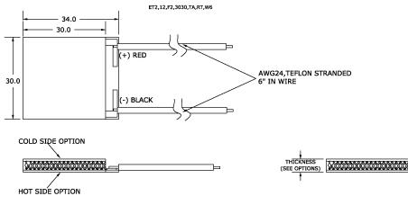
Ceramic Material: Alumina(Al2O3) Solder Construction: 232°C SbSn
