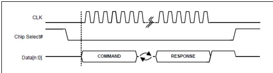
An eSPI transaction consists of a Command phase driven by the master, a turn-around phase (TAR), and a Response phase driven by the slave.
