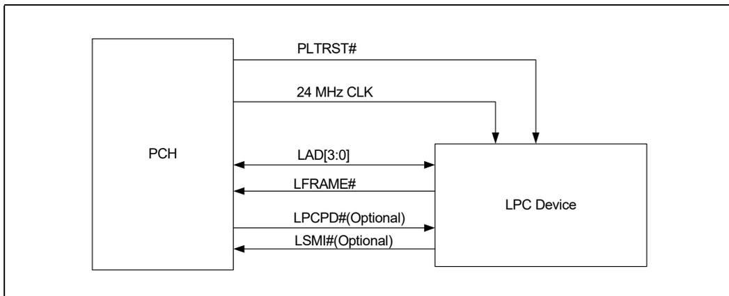
The PCH supports all of the signals that are shown as optional, but peripherals are not required to do so.
