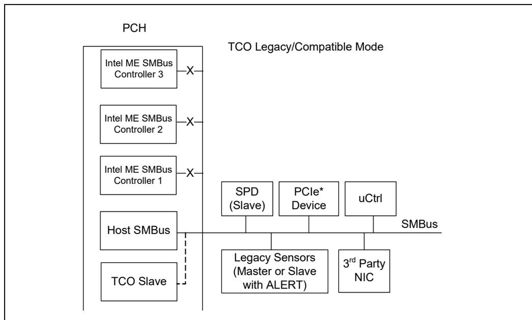
In TCO Legacy/Compatible mode the PCH can function directly with an external LAN controller or equivalent external LAN controller to report messages to a network management console without the aid of the system processor. This is crucial in cases where the processor is malfunctioning or cannot function due to being in a low-power state. Table 5-1 includes a list of events that will report messages to the network management console.
