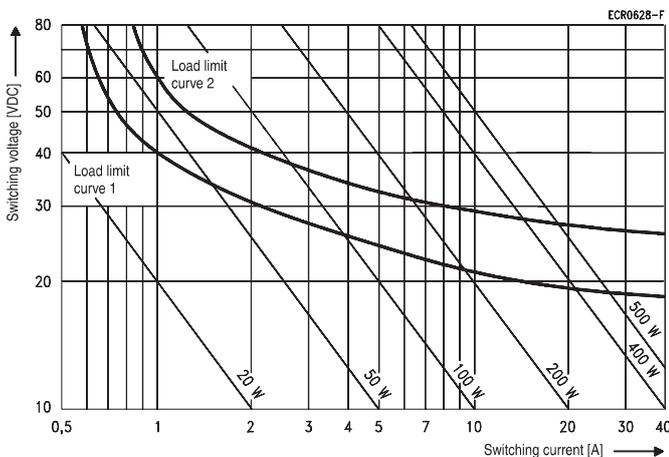
Load limit curve 1: arc extinguishes during transit time (changeover contact).
