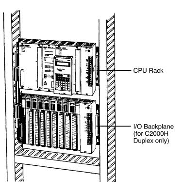
The following figure shows a side view of a mounted CPU and two Expansion I/O Racks. There should be a distance of 70 to 120 mm between the mounted Units.
