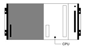
Unlike the CPU of the Package-type PC, the CPU of the Rack PC has no I/O points built in. So, in order to complete this kind of PC we need to mount one or more I/O Units to the Backplane. Mount the I/O Units to the Backplane by pressing the I/O Unit firmly into position, making sure the connectors are properly mated. Secure the Unit by tightening the mounting screws located on the top and bottom of the Unit.
