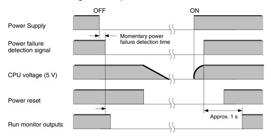
The PC ignores all momentary power failures if the interruption lasts no longer than 10 ms. If the interruption lasts between 10 and 25 ms, the interruption may or may not be detected. If the supply voltage drops below 85% of the rated voltage for longer that 25 ms (less for the DC Power Supply), the PC will stop operating and the external outputs will be automatically turned OFF. Operation is resumed automatically when the voltage is restored to more than 85% of the rated value.
