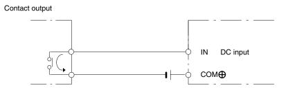
When using the following configurations, the sensor and Input Unit should receive their power from the same supply.
