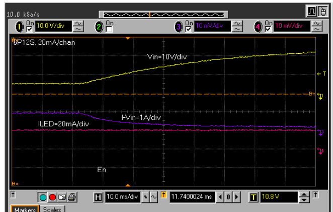
FIGURE 14. LINE REGULATION WITH V_{IN} CHANGE FROM 6V TO 26V, V_{IN} = 12V , 6P12S AT 20mA/CHANNEL
