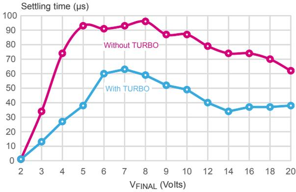
**Figure 7. Settling time from  $V_{START}$  to 2 V**
