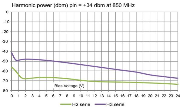
Figure 4. Harmonic power versus bias voltage (shunt)
