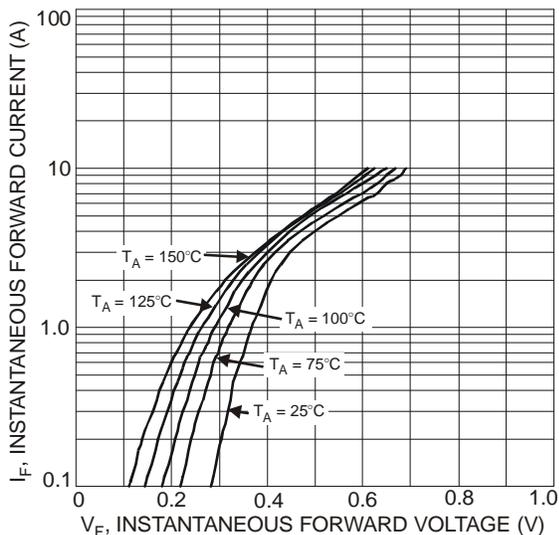
Fig. 1 Typical Forward Characteristics - B320A thru B340A
