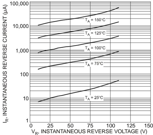
Fig. 3 Typical Reverse Characteristics, B320A thru B340A
