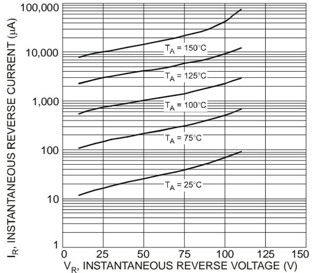
Fig. 4 Typical Reverse Characteristics, B350A thru B360A
