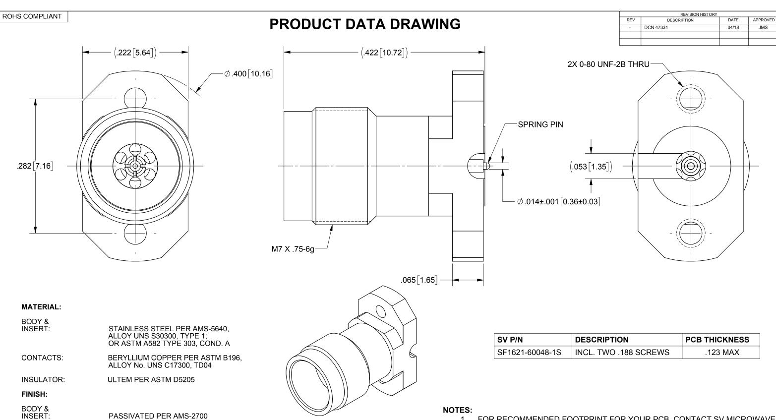
GOLD PER ASTM B488, TYPE II, CODE C, CLASS 1.27, OVER NICKEL PER AMS-QQ-N-290, CLASS 1, .00005" MIN.
