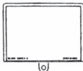
Blank cover In models without a Digital Operator, the blank cover is mounted in place of the Digital Operator.
