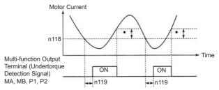
\* Undertorque detection release width (hysteresis) is set at approx. 5 % of the Inverter's rated current.
