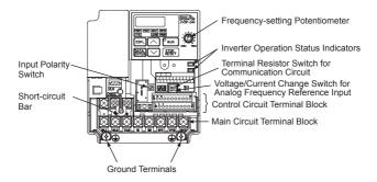
Example for 3-phase (200 V Class, 1.5 kW) Inverter
