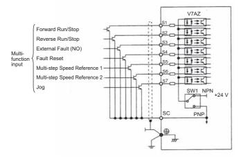
Sequence Connection with PNP Transistor (+24 V Common)
