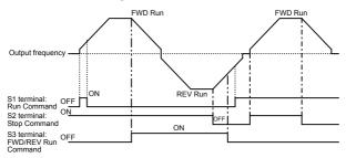
Two-wire Sequence 2 (Special Specifications): Multi-function input selection 1 (constant n050): 1 Multi-function input selection 2 (constant n051): 37 Multi-function input selection 3 (constant n052): Not 0
