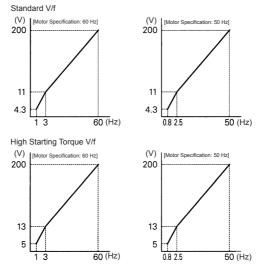
When operating with a frequency larger than 60/50 Hz, change only the Max. Output Frequency (n011).
