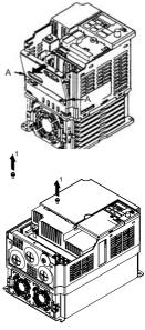
Mounting the Bottom Cover Mount the bottom cover by reversing the order of the above procedure for removal.
