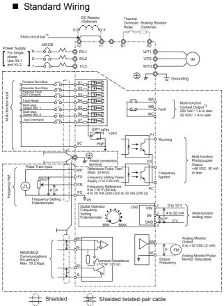
: Only basic insulation (protective class 1, overvoltage category II) is provided for the control circuit terminals. Additional insulation may be necessary in the end product to conform to CE requirements.
