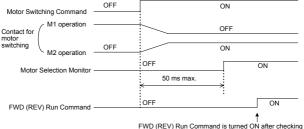
FWD (REV) Run Command is turned ON after checking the status of M1, M2, and the Motor Selction Monitor.
