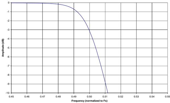
Figure 3. Single Speed Mode Transition Band (Detail)
