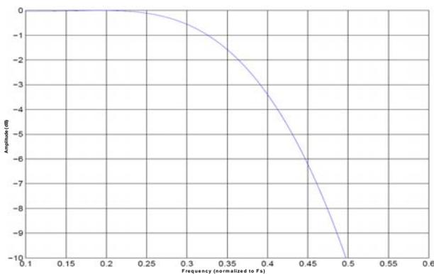
**Figure 11. Quad Speed Mode Transition Band (Detail)**
