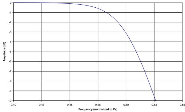
**Figure 7. Double Speed Mode Transition Band (Detail)**
