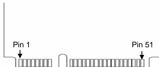
Figure 1-2 Apacer mSATA H1-M pin assignment
