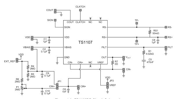
Figure 4.1. TS1107DB Circuit Schematic
