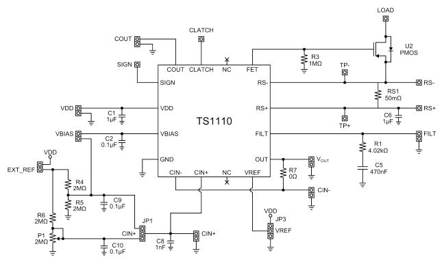
Figure 2.1. TS1110DB Circuit Schematic
