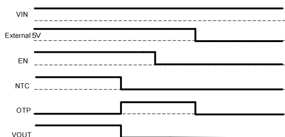
Figure 4: Normal Mode → NTC protection Mode → Transportation Mode
