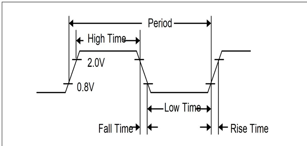
Figure 10-5. Measurement Points for Differential Waveforms
