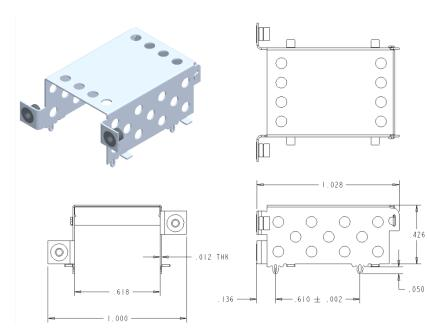
All dimensions in inches. All dimensions +- 0.005", unless noted Screw torque 0.50 +/- 0.10 in-lbs
