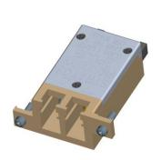
The FNF-LT11 multimode glass optical fiber transceivers provide low profile, cost effective solutions for Fast Ethernet multimode (up to 2.0 km) optical fiber data links with a duplex LC connector interface. These transceivers are fully compliant with the IEEE 802.3u Fast Ethernet standard but can be used for any other data communications purpose within their operating parameters.
