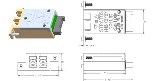
All dimensions in inches. All dimensions +- 0.005", unless noted Screw torque 0.50 +/- 0.10 in-lbs
