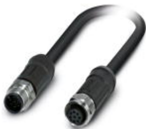
Sensor/Actuator cable, 8-position, PE-X halogen-free, black-gray RAL 7021, Plug straight M12, A-coded, on Socket straight M12, A-coded, Cable length: 2 m, for outdoor applications, with high-grade steel knurl
