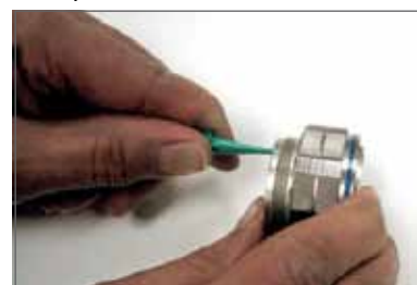
Plastic tool with contact in proper position.
