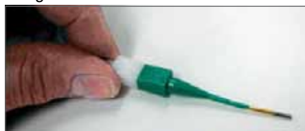
Plastic tool with contact in proper position.
