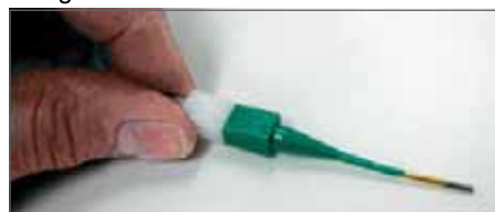
Plastic tool with contact in proper position.
