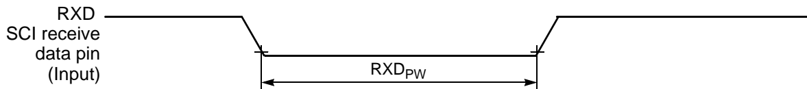
Figure 10-16 RXD Pulse Width
