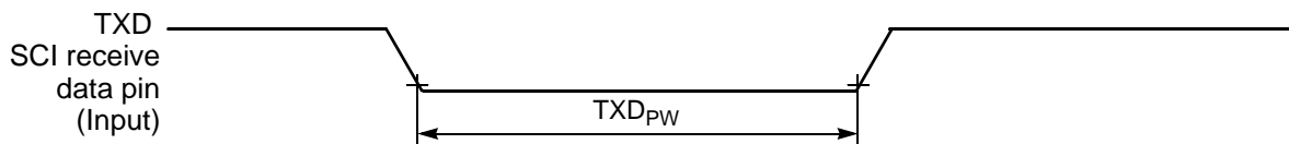
Figure 10-17 TXD Pulse Width
