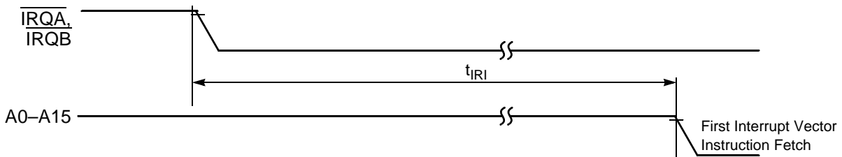
Figure 10-8 Interrupt from Wait State Timing
