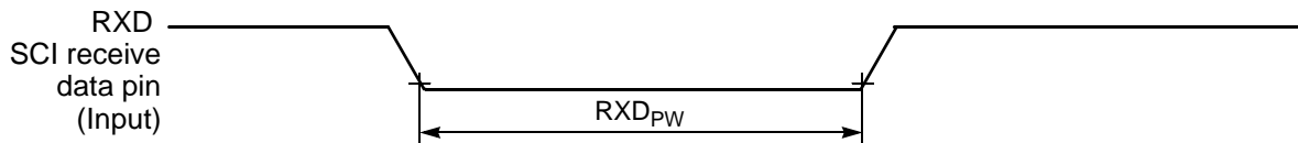
Figure 10-16 RXD Pulse Width
