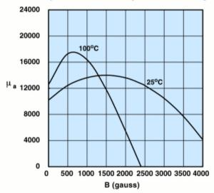
Measured on a 17/10/6mm toroid using the HP 54510A.
