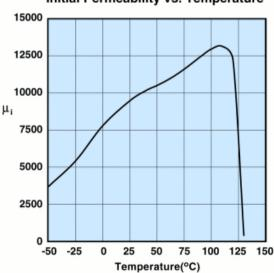
Measured on a 17/10/6mm toroid at 10kHz.
