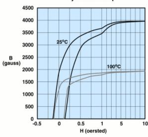
Measured on a 17/10/6mm toroid at 10kHz.
