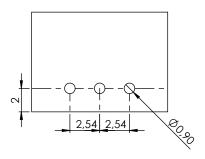
All dimensions in mm. All tolerances  $\pm\,0.5$  mm  $\,$  unless otherwise indicated. Recommended plated drill diameter 0.9 mm.
