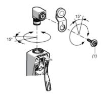
(1) Tightening torque (Min: 1) (Max: 1.5)
