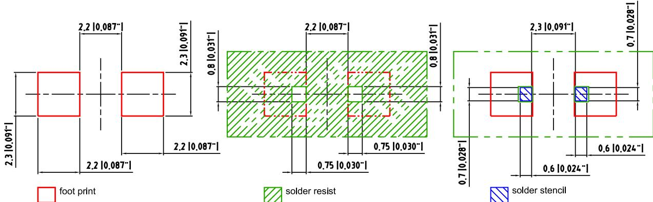
**Component Location on Pad**
