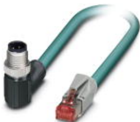
Network cable, Ethernet CAT5, 4-position, PUR, water blue RAL 5021, shielded, Plug angled M12, coding: D, on Plug straight RJ45, cable length: 8.5 m
