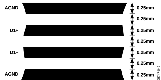
Figure 61. Arrangement of Signal Tracks
