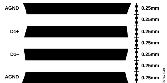
Figure 61. Arrangement of Signal Tracks
