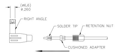
6. ASSEMBLE SOLDER TIP AND CUSHIONED ADAPTER. ALINE THE BANANA PLUG THRU HOLE TO SOLDER TIP. THREAD BY SLIDING SOLDER TIP ASSEMBLY INTO BANANA PLUG THRU HOLE AND TIGHTEN RETENTION NUT TO RIGHT ANGLE.
