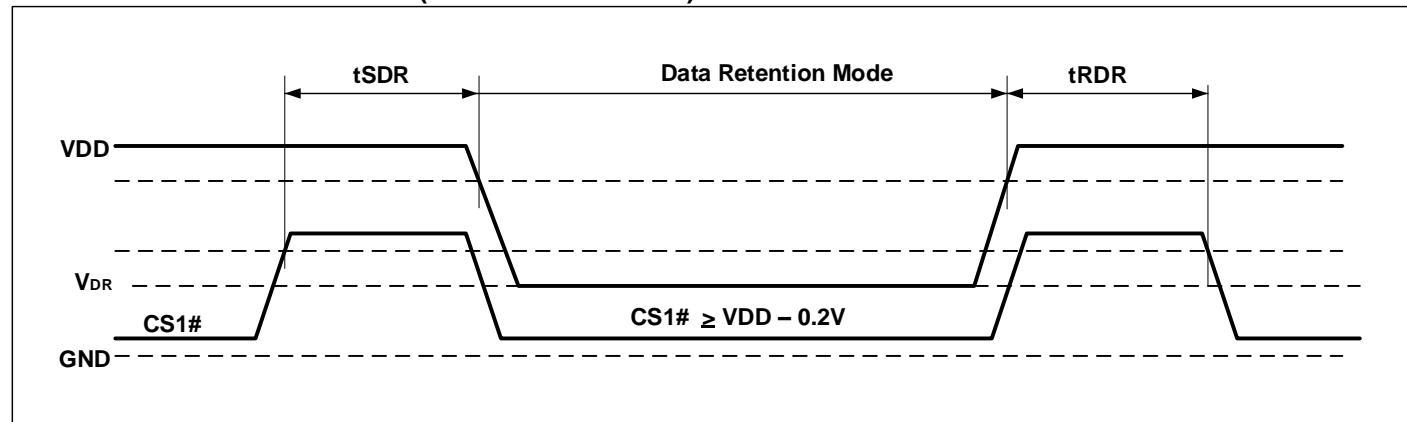
**DATA RETENTION WAVEFORM (CS2 CONTROLLED)**
