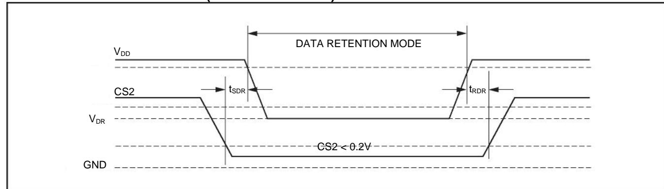
DATA RETENTION WAVEFORM (UB# AND LB# CONTROLLED)
