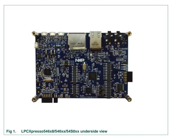
This document describes the hardware of the LPCXpresso546x8/540xx/54S0xx boards, plus information on the CAN-FD shield supplied in the OM13094 kit (this shield board is also available as a standalone product, order code OM13099.) This shield board can be used with any of the LPCXpresso boards described, but note that the LPCXpresso54608 does not support CAN-FD.
