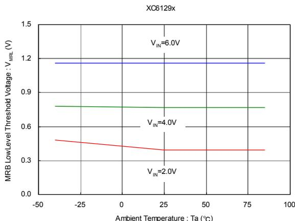
(12) Cd pin MRB Low Level Voltage vs. Input Voltage
