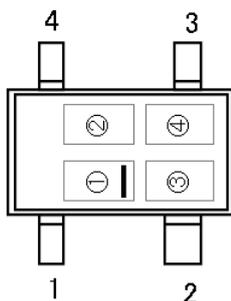
Indicates mark (1) product series. Indicates the detect voltage range and output type.
