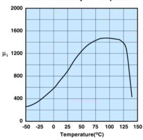
Measured on a 17/10/6mm toroid at 100kHz.
