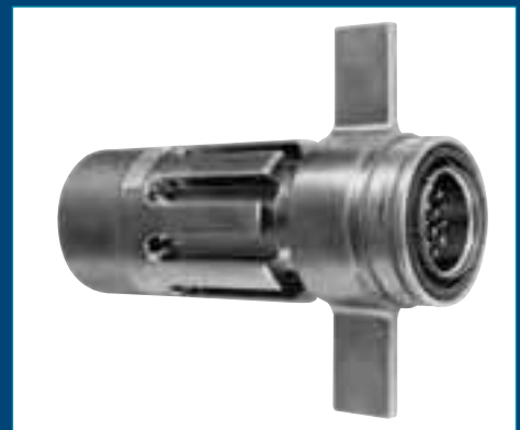
Special configuration Fail Safe used on space telescope application. Lanyard is replaced by a swivel ring for remote disconnect and "wing arms" have been added for manual actuation accessibility by gloved astronauts.
