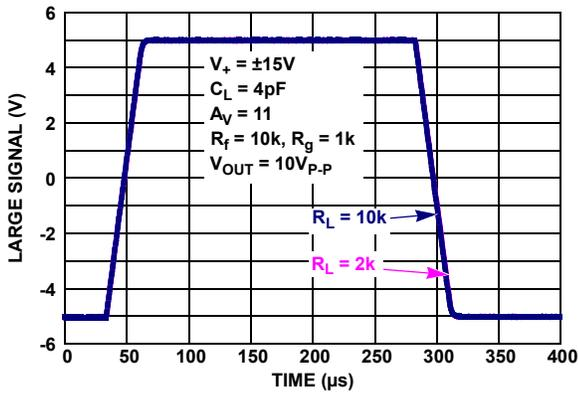
FIGURE 64. CHARACTERIZED LARGE SIGNAL 10V STEP RESPONSE
