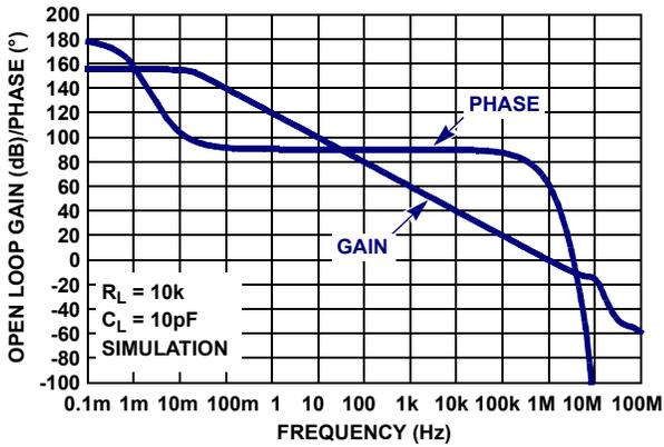
FIGURE 66. SIMULATED OPEN-LOOP GAIN, PHASE vs FREQUENCY
