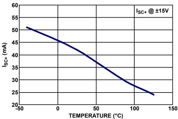
FIGURE 31. POSITIVE SHORT CIRCUIT CURRENT vs TEMPERATURE
