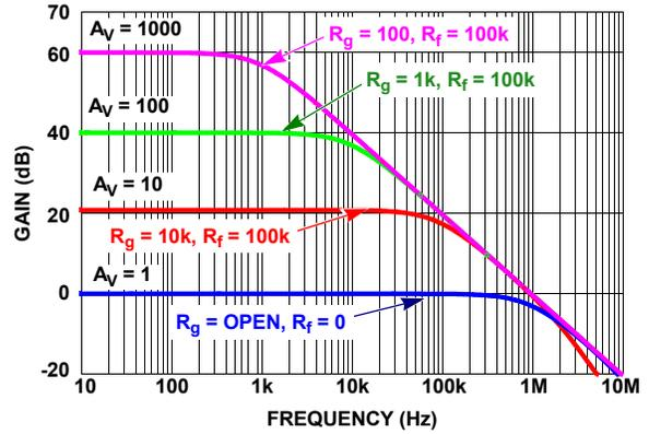
FIGURE 61. SIMULATED CLOSED LOOP GAIN vs FREQUENCY
