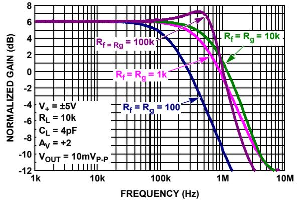
FIGURE 42. FREQUENCY RESPONSE vs FEEDBACK RESISTANCE  $R_f/R_g$
