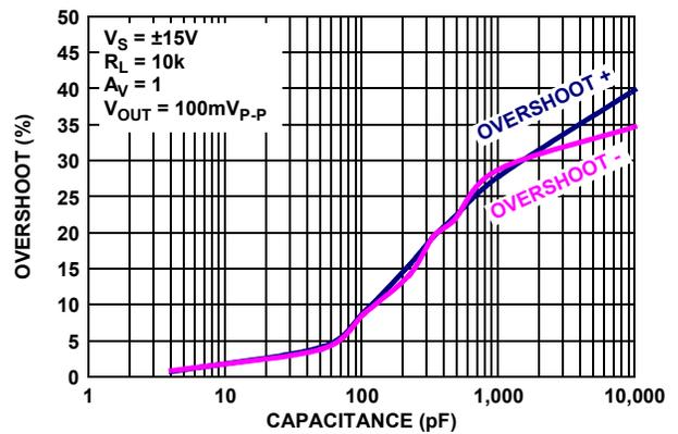
FIGURE 54. % OVERSHOOT vs LOAD CAPACITANCE,  $V_S = \pm 15V$
