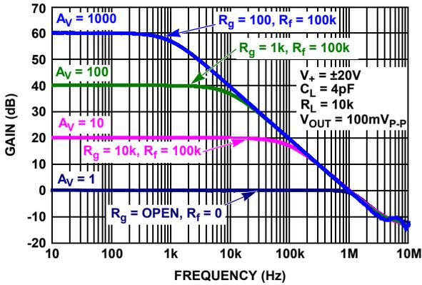
FIGURE 41. FREQUENCY RESPONSE vs CLOSED LOOP GAIN
