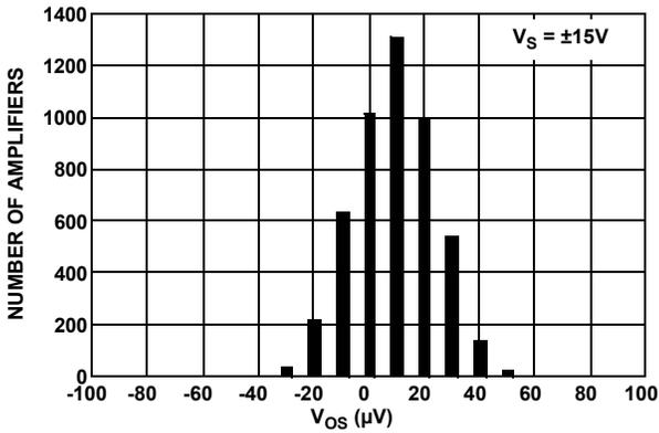
FIGURE 5. INPUT OFFSET VOLTAGE DISTRIBUTION,  $V_S = \pm 15V$
