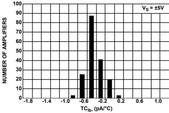
FIGURE 15. TC<sub>1b</sub>-vs NUMBER OF AMPLIFIERS, V<sub>S</sub> = ±5V
