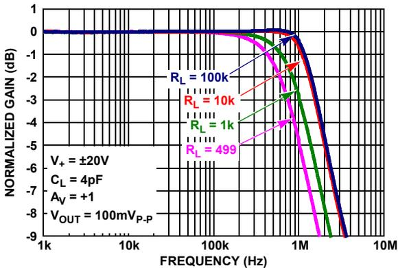
FIGURE 62. CHARACTERIZED CLOSED LOOP GAIN vs  $R_L$
