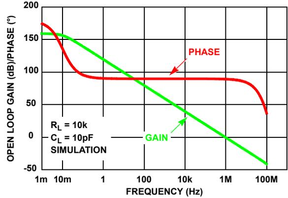
FIGURE 67. SIMULATED OPEN-LOOP GAIN, PHASE vs FREQUENCY
