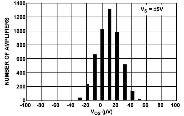
FIGURE 6. INPUT OFFSET VOLTAGE DISTRIBUTION,  $V_S = \pm 5V$
