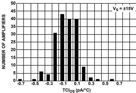
FIGURE 19. TC<sub>1oS-</sub>-vs NUMBER OF AMPLIFIERS, V<sub>S</sub> = ±15V
